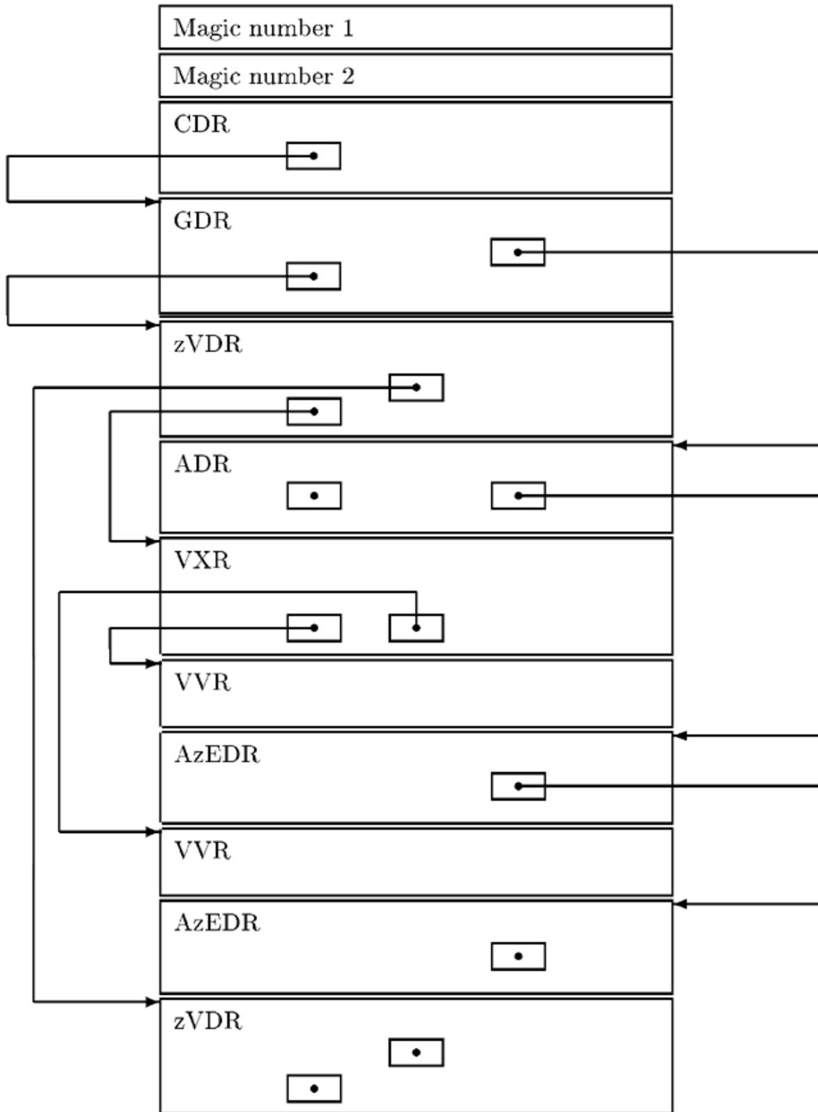
Figure 2.1: Example of an Uncompressed dotCDF File Arrangement
